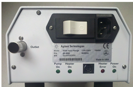
Figure 2 Outlet, Power Switch, LEDs, and Connectors
