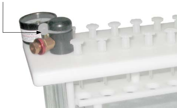
Figure 2. Breaking the vacuum.
