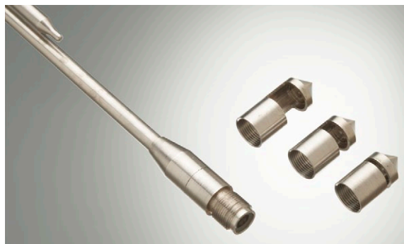
Probes use silica fibers for optimal performance. Interchangeable tips make cleaning and replacement easy. Tip path lengths from 1 to 20 mm are available to accommodate expected absorbance ranges.
