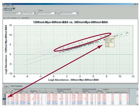
BSA spiked with two different levels of myoglobin simulates a biological sample with differentially expressed proteins. The MassHunter Profiling software clearly identifies myoglobin ions present at different "expression levels." Specific information about each feature is displayed in the feature table and can be displayed in individual pop-up boxes.
