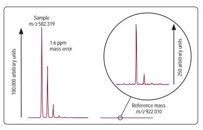
Wide dynamic range ensures that both major and minor components are identified, and facilitates use of an internal standard
