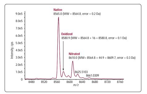
The MassHunter Bioconfirmation software discerns modified forms of proteins, as shown in this deconvoluted spectrum of three major products in a peroxynitrite-treated ubiquitin sample
