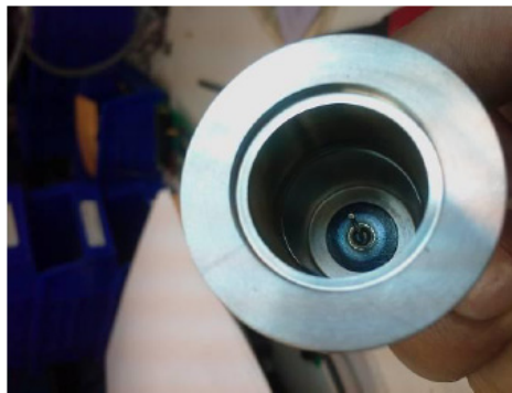
Figure 2-4 Clean Collector Chamber
