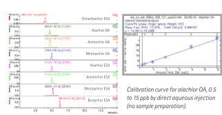
MRM chromatograms of the six regulated Method 535 analytes at 1 ppb.
