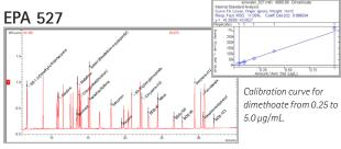
Full Scan EI/MS TIC of Method 527 pesticides and polybrominated diphenylethers (PBDEs) at  $5 \mu g/mL$ .
