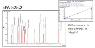
Full scan EI/MS TIC of all regulated Method 525.2 targets along with the new UCMR2 analytes (alachlor, acetochlor, metolachlor) at  $5\,\mu g/mL$ .
