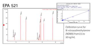
GC/MS/MS total ion chromatogram (TIC) of all EPA Method 521 target analytes at 50 ng/mL. Note the excellent linearity, chromatographic peak shape, and resolution.
