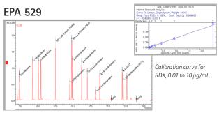
Full scan EI/MS TIC of all target explosives at a concentration of  $2 \mu g/mL$ .
