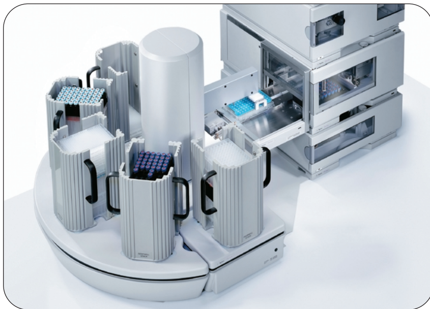
Figure 7 Sample capacity extension and well-plate handler of the Agilent 1100 Series high throughput LC/MS system leading to a sample capacity of up to 30,720 samples.
