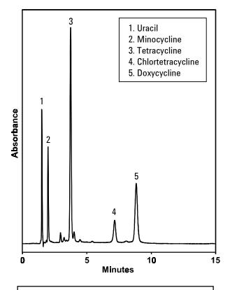
Conditions: ZORBAX Rx-C8 (4.6 x 150 mm) (Agilent P/N: 883967-901) Mobile Phase: 75:25 0.1% TFA : Acetonitrile 1.0 mL/ min, Ambient, Detect. UV (254 nm)
