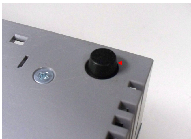
Figure 8: Adhesive Rear Feet Installed
