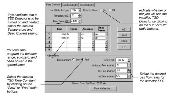
The first row of the spreadsheet contains the Initial Range, Autozero, and Bead Power settings for the TSD Detector. The TSD will switch to this setting when the method is activated, and will be restored to this setting when each chromatographic run is completed.
