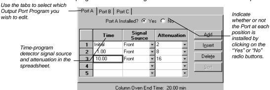
The first row of the spreadsheet contains the Initial Signal Source and Attenuation for the Port. The Port will switch to this setting when the method is activated, and will be restored to this setting when each chromatographic run is completed.
