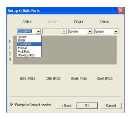
After you have completed your selections, the Setup COMM Ports Dialog should appear similar to the following figure. The selected serial port is dedicated to the CPAL and should not be used to connect any other serial device.
