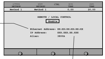
Use the Ethernet address shown here when setting up the BOOTP Server.
