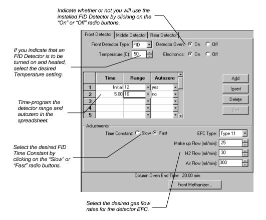
The first row of the spreadsheet contains the Initial Range and Autozero for the FID Detector. The FID will switch to this setting when the method is activated, and will be restored to this setting when each chromatographic run is completed.
