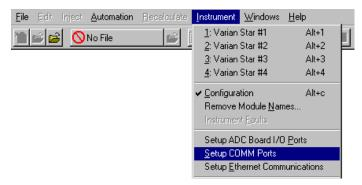
If the Combi PAL driver is installed, 'CombiPAL' is one of the choices available from the drop-down box below each available Serial COMM port. Select "CombiPAL" in the drop-down box below the port in which the 9-pin cable is attached to the Workstation's RS232 port (COM1-COM4).
