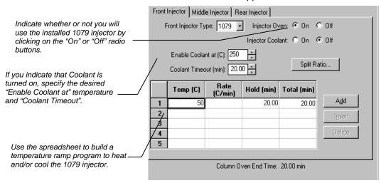
The first row of the spreadsheet contains the Initial temperature and hold time for the 1079 injector. The 1079 will equilibrate to this setting when the method is activated, and will be restored to this setting when each chromatographic run is completed.
