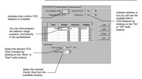
The first row of the spreadsheet contains the Initial Range, Autozero, and Polarity for the Micro-TCD Detector. The Micro-TCD will switch to this setting when the method is activated, and will be restored to this setting when each chromatographic run is completed.
