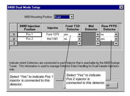
A SampleList for the 8400 AutoSampler or the 8410 AutoInjector will have a column labeled "Injectors Used". For Dual Mode injections, you need to select both injectors.
