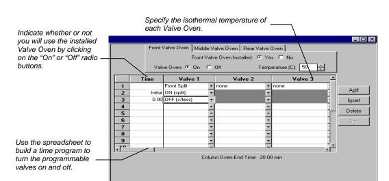
If you indicate that a Valve Oven is installed, a Valve Oven switch and a Temperature setting will appear.
