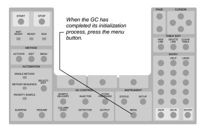
The Instrument menu is displayed. Press 1 to select the Remote/ Local Control screen. The Ethernet address, IP address and Alias (which may not yet be assigned) are displayed.
