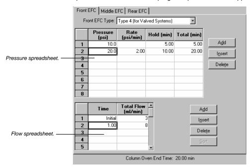
The first row of the pressure spreadsheet contains the Initial pressure and hold time for the Type 4 EFC. The EFC will equilibrate to this setting when the method is activated, and will be restored to this setting when each chromatographic run is completed.
