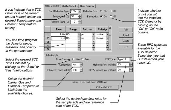
The first row of the spreadsheet contains the Initial Range, Autozero, and Polarity for the TCD Detector. The TCD will switch to this setting when the method is activated, and will be restored to this setting when each chromatographic run is completed.
