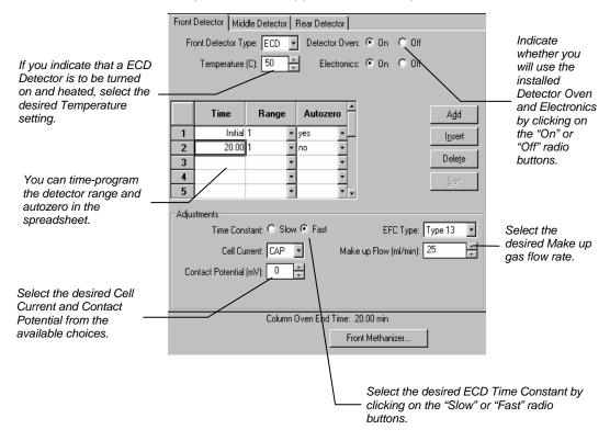
The first row of the spreadsheet contains the Initial Range and Autozero for the ECD Detector. The ECD will switch to this setting when the method is activated, and will be restored to this setting when each chromatographic run is completed.
