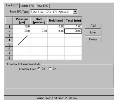
Use the spreadsheet to build a pressure ramp program to control the Type 1 EFC.
