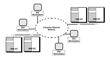
We refer to this type of multi-purpose network as a *company network*, and it will typically be managed by a Network Administrator in your company. If this is the case, then follow the instructions for configuring your 3800 GC and Workstation for use on a company network.
