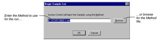
After you click on **OK**, the Method is downloaded to the 3800 GC and the run will begin. If you are using a manual injector or a sampling device that is not controlled by the Star Workstation, you will need to start the device manually.
