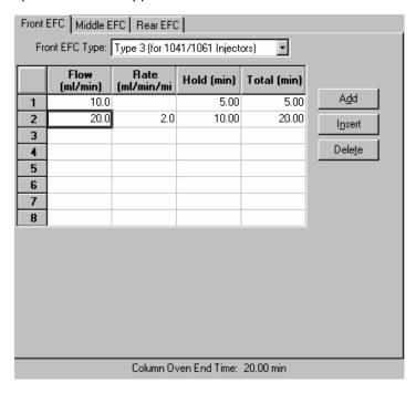
The first row of the spreadsheet contains the Initial flow and hold time for the Type 3 EFC. The EFC will equilibrate to this setting when the method is activated, and will be restored to this setting when each chromatographic run is completed.
