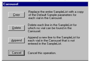
The SampleList is then updated with the vial information from the AutoSampler. Default values are used for each entry added to the SampleList. Refer to the 8200/SPME AutoSampler for 3800 GC Manual for details about use of the 8200 AutoSampler with the 3800 GC.
