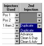
If "Duplicate" is selected, upon finishing the 1<sup>st</sup> injection the 8400/8410 will immediately proceed to withdraw sample from the vial and perform the 2<sup>nd</sup> injection. If "Clean & Dup" is selected, upon finishing the 1<sup>st</sup> injection the 8400/8410 will clean the syringe with wash solvent before proceeding with the 2<sup>nd</sup> injection.
