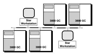
We refer to this type of special purpose network as an *isolated network* (one that does not have IP addresses prescribed by a Network Administrator).
