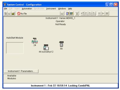
There can only be a single Combi PAL assigned to each instrument. If you wish the AutoSampler to begin sampling automatically when automation is started, place the Combi PAL icon in the AutoStart Module box for the Instrument. System Control will remember where to put the icon the next time that the AutoSampler connects.
