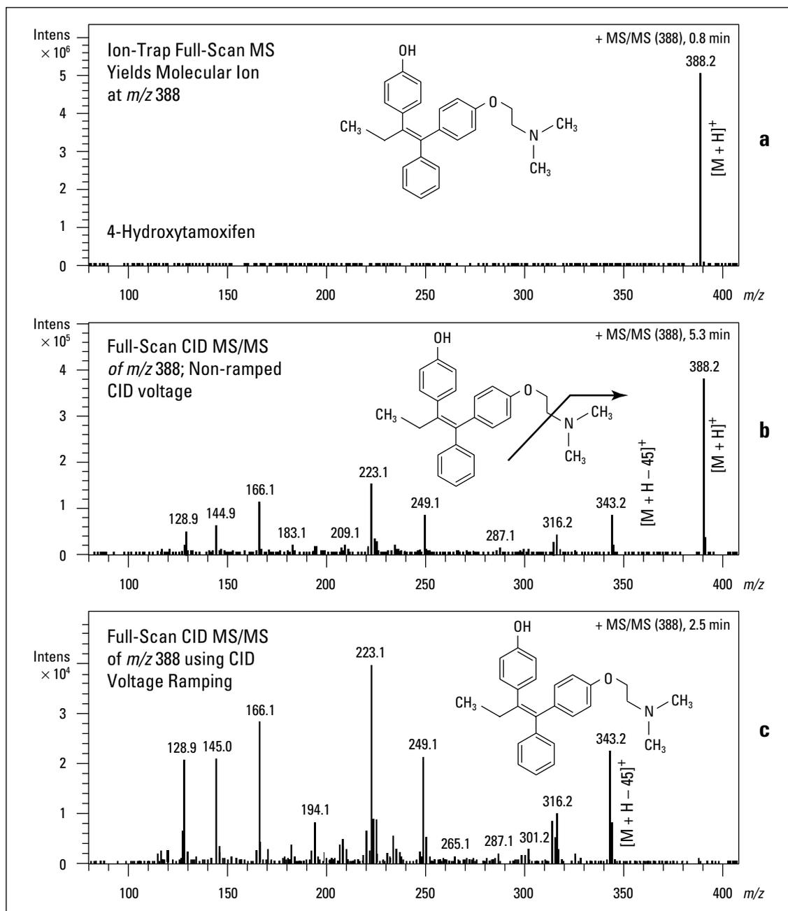
Figure 3. MS/MS of 4-hydroxytamoxifen using CID voltage ramping
