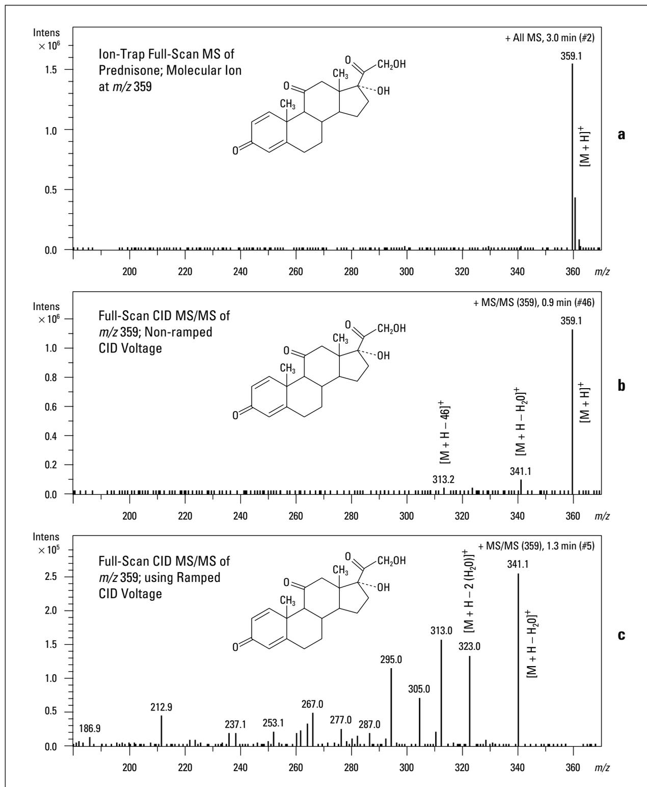
Figure 1. MS/MS of Prednisone using CID voltage ramping
