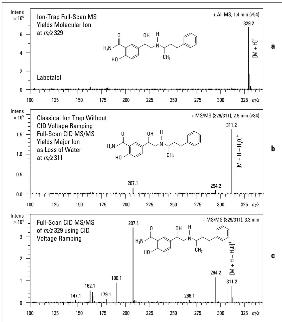
Figure 2. MS/MS of Labetalol using CID voltage ramping
