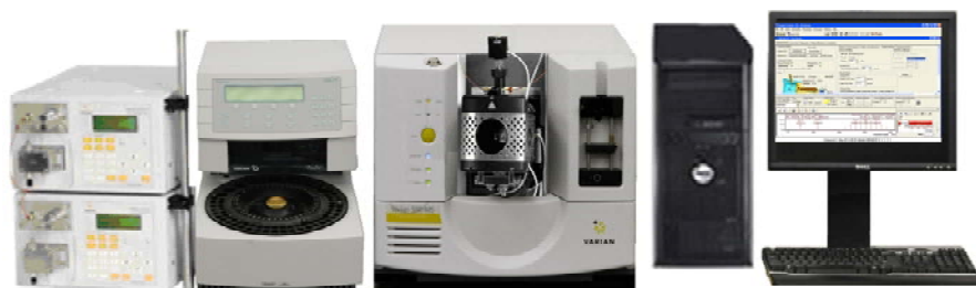
Figure 1 Typical Layout of the 500-MS with the 212-LC pumps
