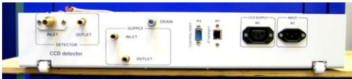
Figure 5.2.1 Electrical and Water Connections on the Back of the KMW200B
