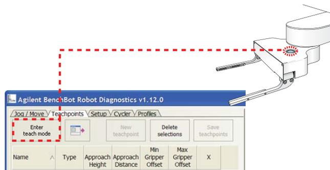
You should be able to move the robot arm without resistance.
