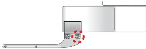
The washers are used to ensure the tips of the grippers point slightly inward to ensure optimal grip performance. The following diagram exaggerates the inward positioning.
