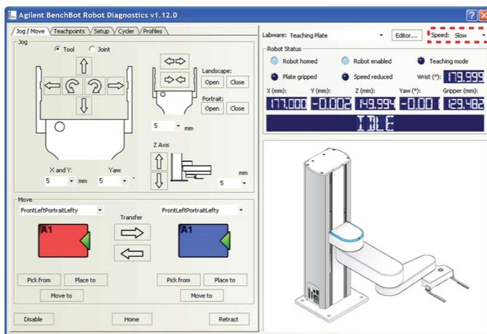
*Note:* During a protocol run, the robot will use the speed selection in the VWorks software Tools > Options dialog box. If the robot is holding a microplate, the slower of the following will be applied: the speed for the selected labware in the Labware Editor or the speed in the Tools > Options dialog box. For more information, see the [VWorks Automation Control Setup Guide](#) and [VWorks Automation Control User Guide](#).
