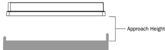
You can reduce the Approach Height value to prevent collision with shelves or other obstacles above the teachpoint. However, make sure there is sufficient clearance below the labware to prevent collision with raised tabs or other obstacles at the teachpoint.
