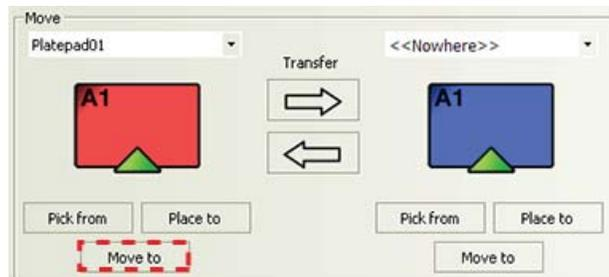
The robot moves to the selected teachpoint. The robot remains at the teachpoint and the grippers are open.
