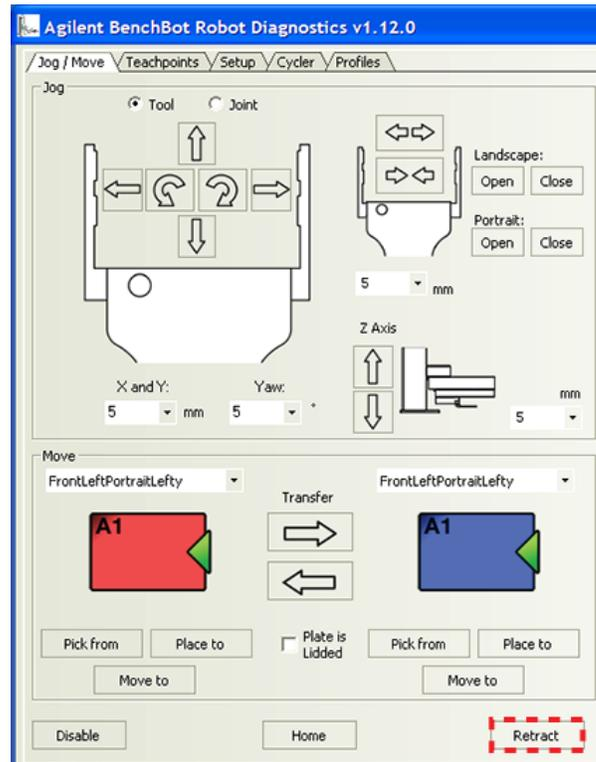
The robot searches for the closest teachpoint, and then uses the approach distance from that teachpoint to retract into the robot zone. If the robot is unable to find a teachpoint nearby, it will retract directly into the robot zone.
