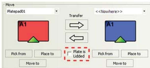
**IMPORTANT** The sum of the grip height plus the finger height must be less than the lid-resting height (specified in the Labware Editor). Otherwise, the software will display an error message when you attempt to pick up the labware with lid.
