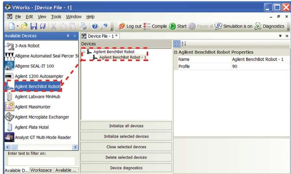
Notice that the first BenchBot Robot device is labeled BenchBot Robot-1. If you add another BenchBot Robot device, it will appear as BenchBot Robot-2.
