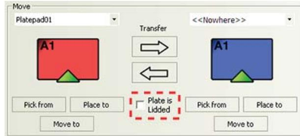
**IMPORTANT** The sum of the grip height plus the finger height must be less than the lid resting height (specified in the Labware Editor). Otherwise, the software will display an error message when you attempt to place the labware with lid.
