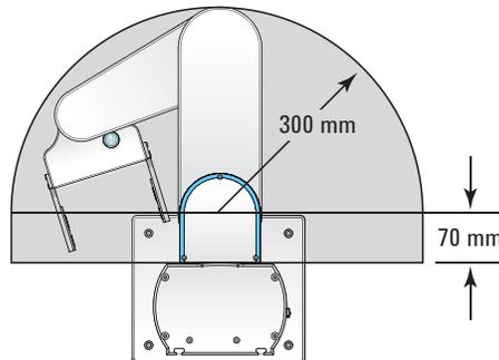
You can retract the robot into the robot zone. Retract the robot into the robot zone when:
