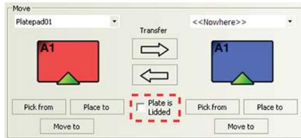
**IMPORTANT** The sum of the grip height plus the finger height must be less than the lid resting height (specified in the Labware Editor). Otherwise, the software will display an error message when you attempt to pick up or place the labware with lid.
