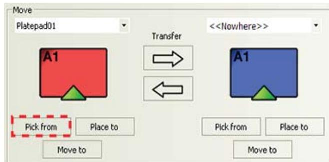
The robot moves to the teachpoint, picks up the labware, and moves it to the robot zone. The labware remains in the robot grippers.
