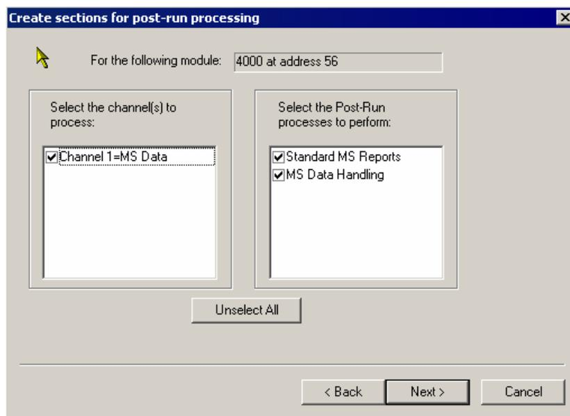
The method will contain the following sections: 3800 GC Control, 4000 MS Control, Standard MS Reports and MS Data Handling.
