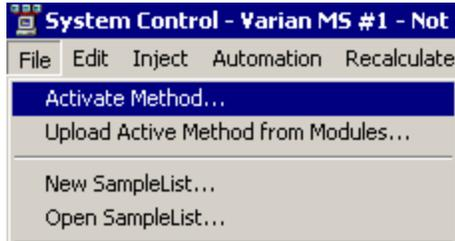
Choose a method and click **Open**. The new GC/MS method will be downloaded to the instrument. The eight most recent methods are available under the **Recent Files** button (see below).
