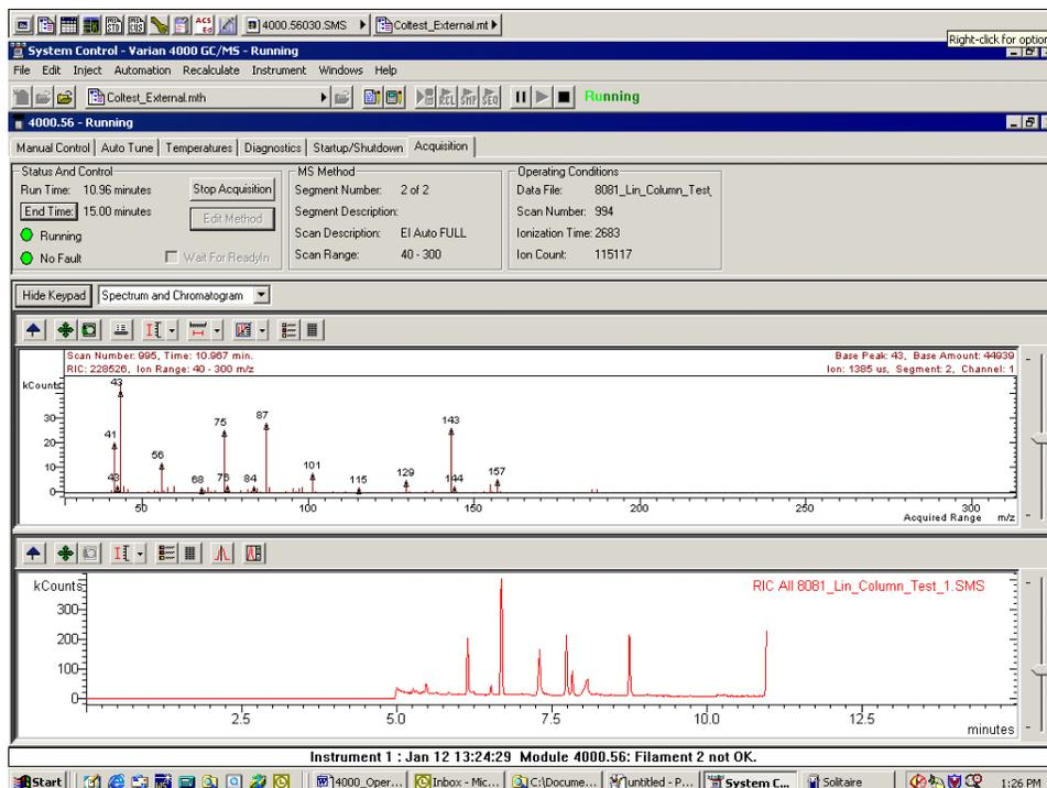
The module status is shown in the status and control windows and on the Toolbar. You can monitor the chromatogram and spectra here in System Control, or you can click the far right button in the Chromatogram toolbar to transfer to MS Data Review, where you can perform operations like library searching while the data file is being acquired.
