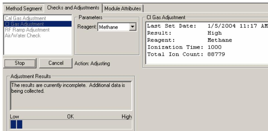
Highlight **CI Gas Adjustment** and click the **Start** button. Use the CI Gas Adjust Valve (#3) inside the front door of the 4000 MS. Turn the knob clockwise to increase the flow or counterclockwise to decrease the flow. The objective is to set the ion gauge pressure within the range of 70 – 100  $\mu$ Torr.
