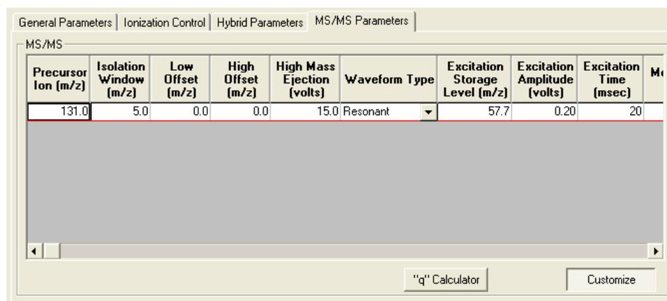
**Precursor Ion (m/z):** The precursor ion is the desired ion m/z that will be isolated in the MS/MS isolation step. This Precursor Ion m/z value is used in both Resonant and Non-Resonant Methods of MS/MS.
