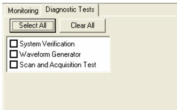
After the turbomolecular pump reaches 100% speed, you can begin normal operations with the MS. It is a good idea to check for instrument problems by running all of the routines in the Diagnostic Tests tab dialog of the Diagnostics mode. Click the **Select All** button and then click the **Start Diagnostic** button in the Control and Status field to the left. If a test fails, refer to the relevant section of the Troubleshooting Guide in the 4000 GC/MS Hardware Operation Manual.
