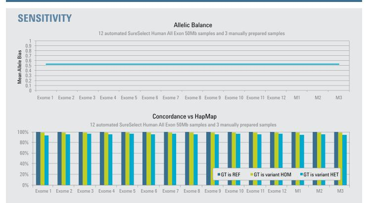
The Automated SureSelect Library Prep and Capture System maintains excellent allelic balance, strong concordance and sensitivity versus HapMap samples allowing you to process samples with the confidence of manual SureSelect preparations and ease of automation. Genotype (GT) reference (REF) match reported sequence and are captured at > 99.9% efficiency. Homozygous (HOM) and heterozygous (HET) variants are captured with equally high efficiency at > 97%.
