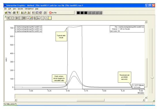
Here a threshold of 25000 microAU is used to detect the presence of a peak and start the ratioing process. Note that the cursor in Interactive Graphics is set at the start of the ratio and the signal reading is 25 mAU (25000 microAU).
