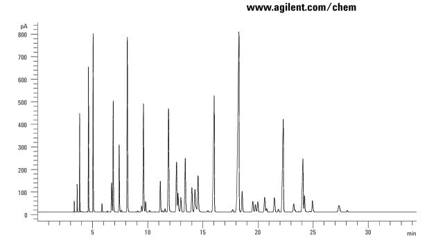
Chromatogram shows naphtha cut up to C9.
