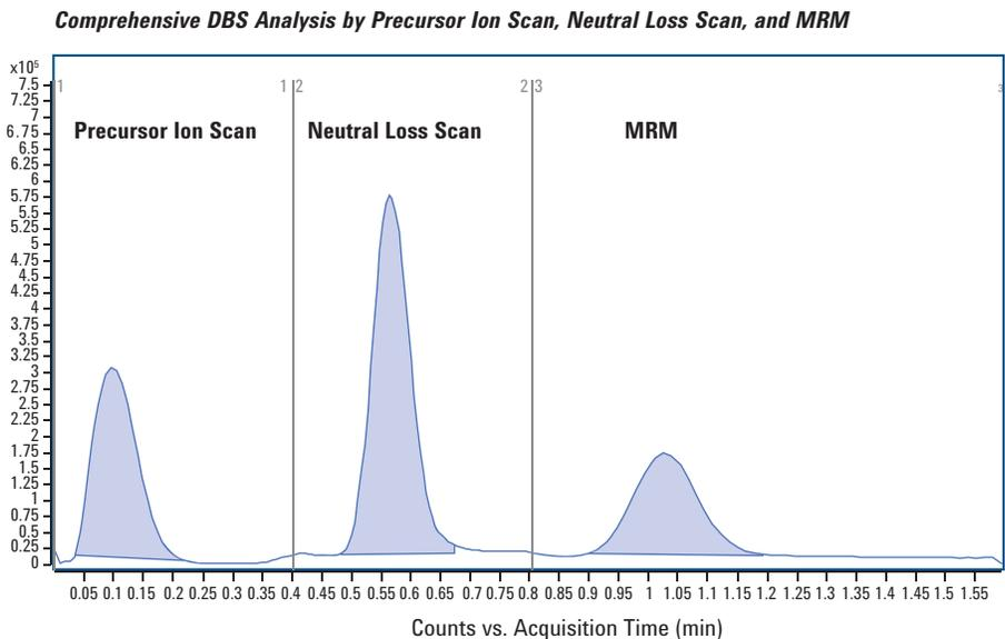
Figure 1. Reconstructed Total Ion Current Chromatograms (RTICC) showing the three sequential scans run on the same dried blood spot sample.
