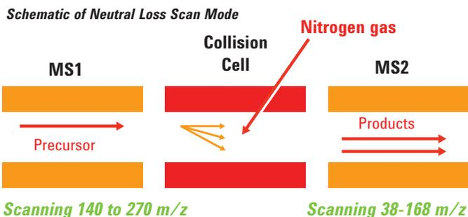
Figure 2. The first quadrupole mass analyzer (MS1) and third quadrupole (MS2) are set at a fixed difference (102 Da) in the mass-to-charge ratio ( $m/z$ ) while both are scanning over a user-defined mass range (MS1: 140 to 270; MS2: 38 to 168).
