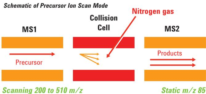
Figure 4. The first quadrupole mass analyzer (MS1) scans over a defined mass range of 85 to 200, while the second quadrupole (MS2) is fixed to detect only product ions of  $m/z$  85. The combination of a specific precursor  $m/z$  with the product ion  $m/z$  of 85 is characteristic for each acylcarnitine.
