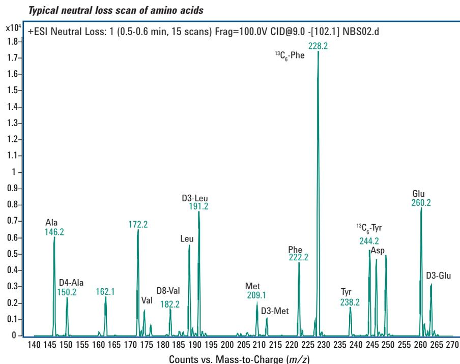
Figure 3. Neutral Loss Scan of 102  $m/z$  for amino acids.
