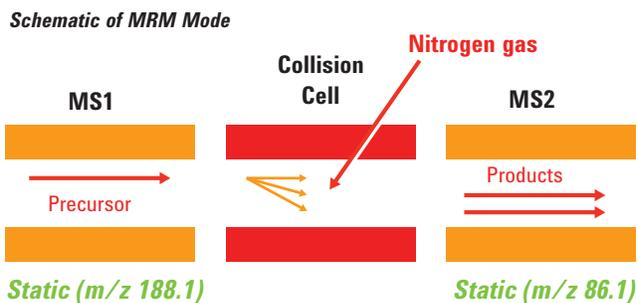
Figure 6. Both the first (MS1) and third quadrupole (MS2) mass analyzers are held static at the mass-to-charge ratios ( $m/z$ ) of the precursor ion and the most intense product ion, respectively, characteristic of a particular amino acid or acylcarnitine, in this case.
