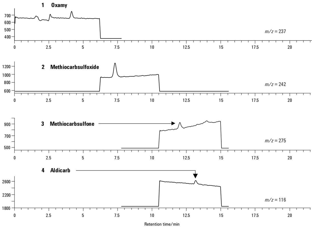
**Figure 3. SIM chromatograms of four carbamate standards at 0.2 ppb. The base peak is labeled in each chromatogram.**
