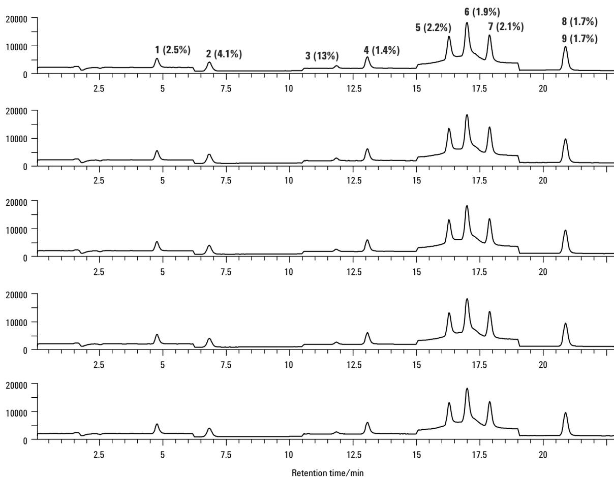
**Figure 7.** Repeatability of five repeat injections of the carbamate standards at 5 ppb. The percentage number in each parenthesis is the %RSD value for the peak.
