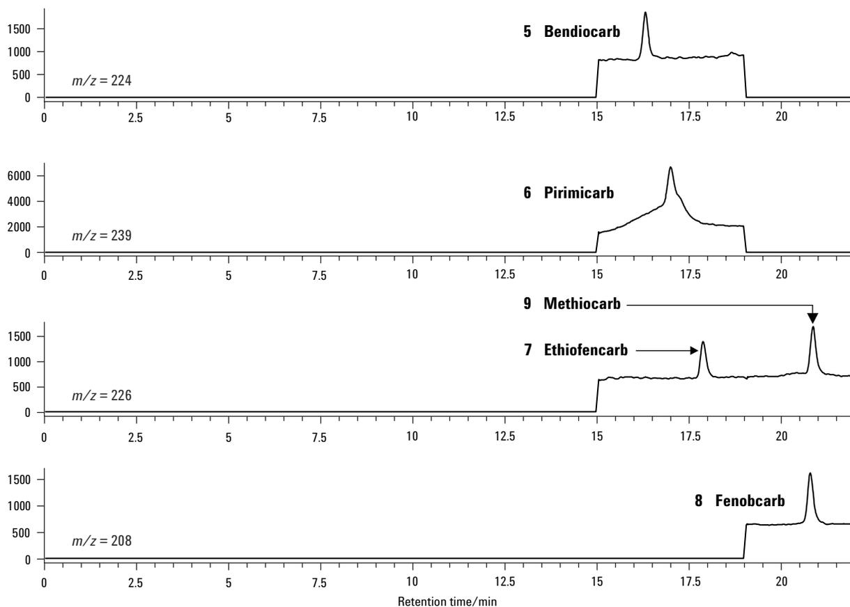
**Figure 4. SIM chromatograms of five carbamate standards at 0.2 ppb. The base peak is labeled in each chromatogram.**
