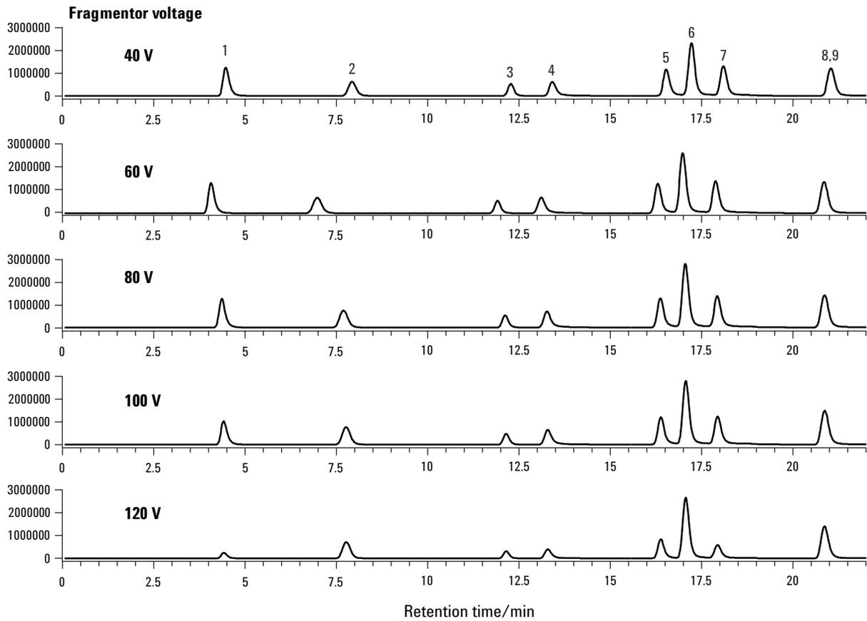
Figure 5 SIM chromatograms of carbamate standards at different fragmentor voltages.
