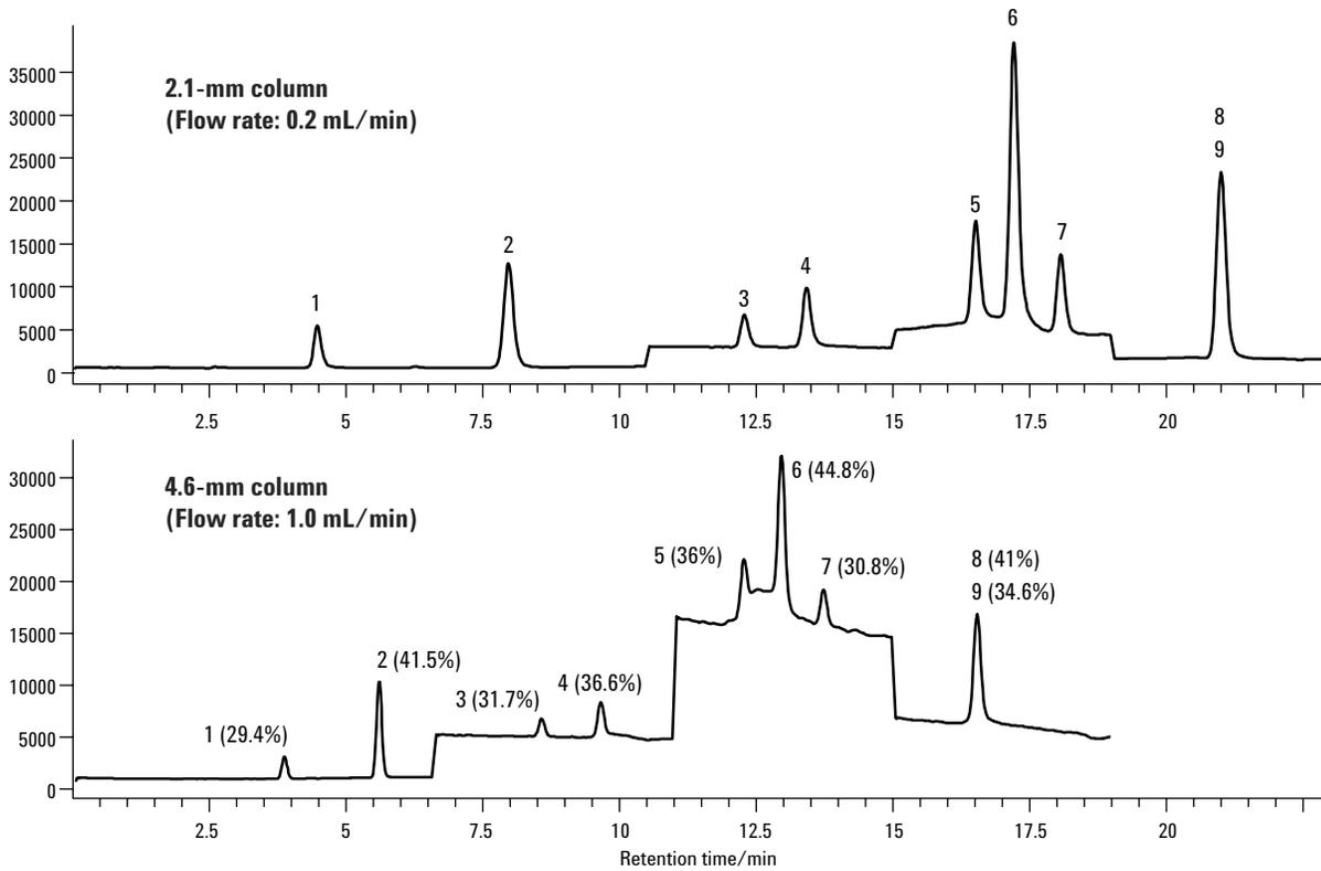
**Figure 9.** Comparison of 10-ppb chromatograms on a 2.1-mm column and a 4.6-mm column. The percentage number in each parenthesis is the relative response of the analyte from the 4.6-mm column to the peak intensity from the 2.1-mm column.
