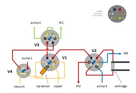
Figure 5 Flush the sipper tube
