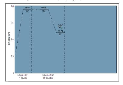
Run the PCR<br/>Program1Place the reactions in the Mx3000P/Mx3005P instrument.2On the Run screen, click Start Run.
