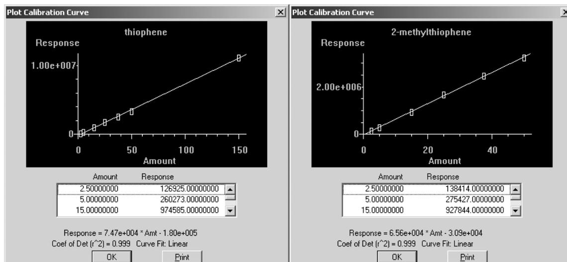
Figure 2. Calibration curves, thiophene and 2-methylthiophene in 3:1 isooctane:toluene.
