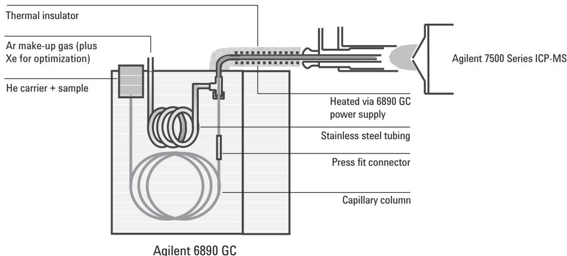
Figure 1. Schematic diagram of Agilent GC-ICP-MS system.
