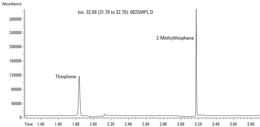
**Figure 7. Calibration standard, 2.5 ppm each thiophene and 2-methylthiophene.**
