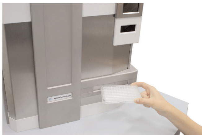
Figure 2. Inserting a crystallisation plate into the PX Scanner.
