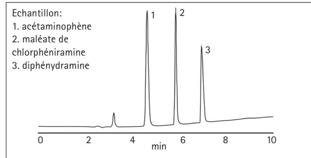
Colonne: Pursuit XRs-C18 10 µm, 250 x 4,6 mm, Phase mobile: A: H<sub>2</sub>O + 0,1% HCOOH, B: CH<sub>3</sub>CN + 0,1% HCOOH, Gradient: 15-70% B en 10 min, Débit: 1,0 mL/min, Temp.: ambiante, Détection: UV @ 254 nm
