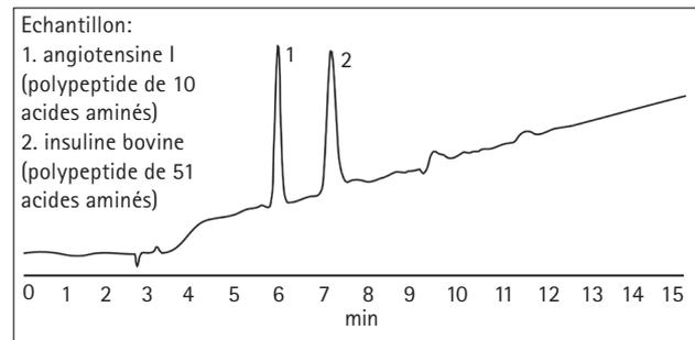
Colonne: Pursuit XRs-C18 10 µm, 250 x 4,6 mm, Phase mobile: A: H<sub>2</sub>O + 0,1% TFA, B: 80% CH<sub>3</sub>CN + 0,1% TFA, Gradient: 30-80% B en 15 min, Débit: 1,0 mL/min, Temp.: ambiante, Détection: UV @ 215 nm
