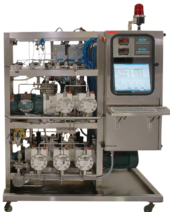
SepTech 2.5 L/min. XP/EX high pressure Skid system with temperature control and Steady-State recycle technology
