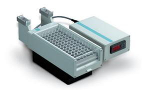
The Peltier-cooled trayholder is ideal for thermally labile samples.
