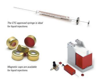
You can use an injector and heater module for headspace sampling.
