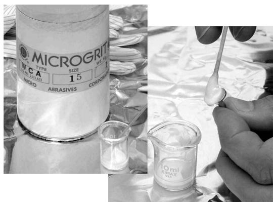
**Figure 4. Microgrit and slurry.**
