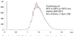
Fast simulated distillation of cracked gas oil in less than 3 minutes — 6x faster than conventional ASTM D2887 GC procedure—using a temperature ramp of 150°C/min. Chromatographic overlay of 10 runs shows outstanding repeatability. (2)
