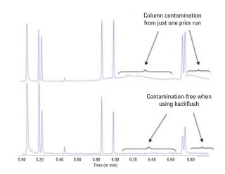
**Backflushing.** In this polynuclear aromatic hydrocarbons (PAH) analysis by LTM/GC/MS, the upper chromatogram shows that even after one run, soil extracts can contaminate the column, causing baseline increases that affect subsequent runs.
