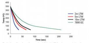
**Typical cooling times** for standard (5-inch) LTM column modules of typical lengths are significantly faster than a conventional GC oven.
