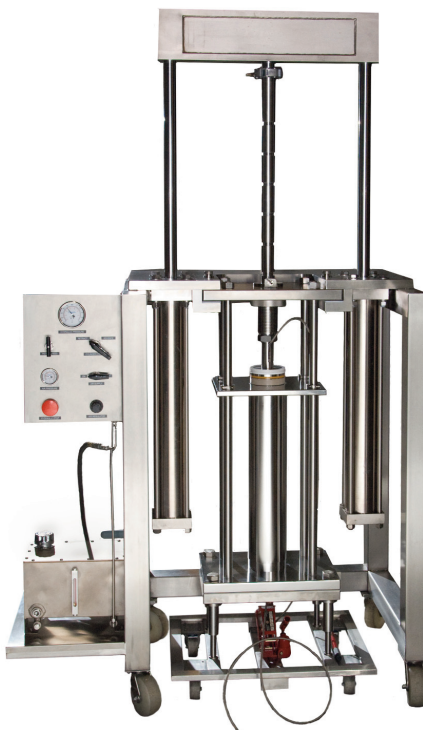
Removal of the sorbent by plunger extension to ease the unpacking process and minimize handling of sorbent and solvents.
