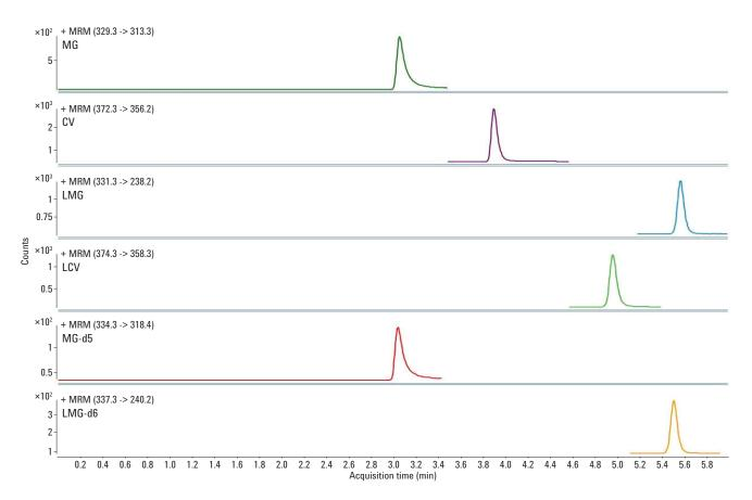
Figure 2. Chromatograms of 10 ng/g spiked sample extracts of antibacterial agents in fish on an Agilent Poroshell 120 EC-C18 column
