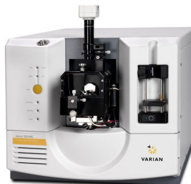
Figure 4. Varian 500-MS ion trap mass spectrometer with nESI.
