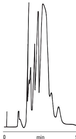
Figure 3. Isocratic separation of 0.92 mg of crude synthetic ACP 65-74 using a PLRP-S 100Å analytical column.
