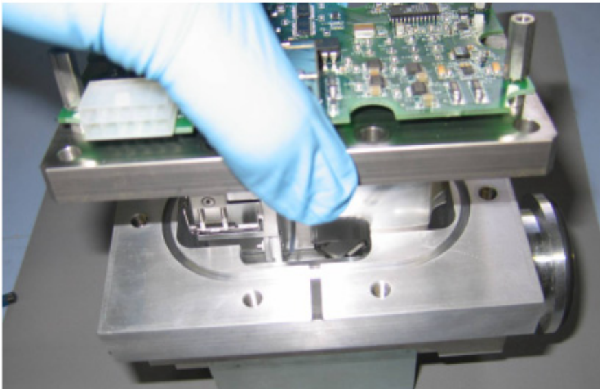
Figure 7: Spectrometer Assembly Removal
