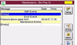
Maintenance shows the logs for maintenance related events, and allows access to EMF (early maintenance) settings and functions needed for maintenance tasks (e.g. calibration routines, parts information).
