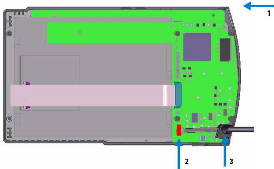
Figure 118 Rear Panel - location of cable, connector and release button
