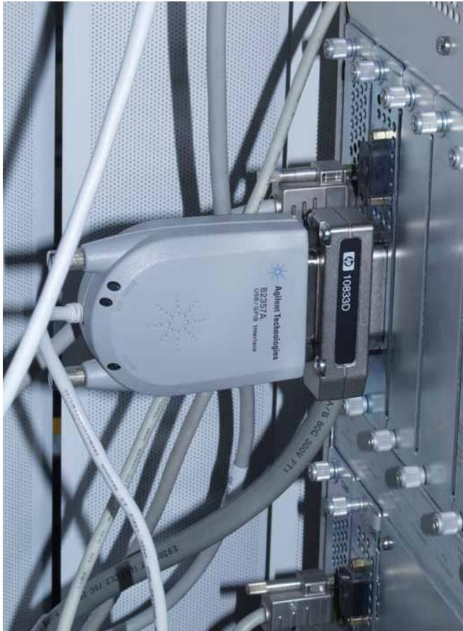
**Figure 14** 82357A USB-GPIB Interface on e.g. HP 1090/DAD
