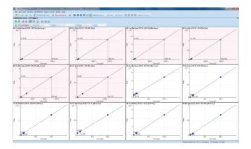
Calibration curves can be shown as a summary (12 plots, shown above), or as individual plots. Elements with an outlier flag for the current sample are also highlighted (red shading) in the calibration plots.
