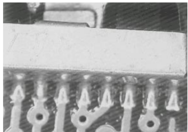
Picture 4. Unit self-aligns after reflow.
