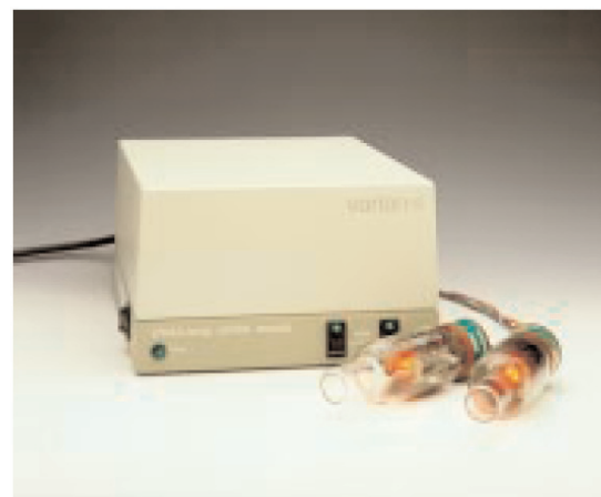
Figure 6. The additional boosting circuit requires its own power supply.
