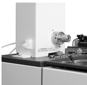
Agilent pneumatic air actuator/valve assembly installed on the 7890A.
