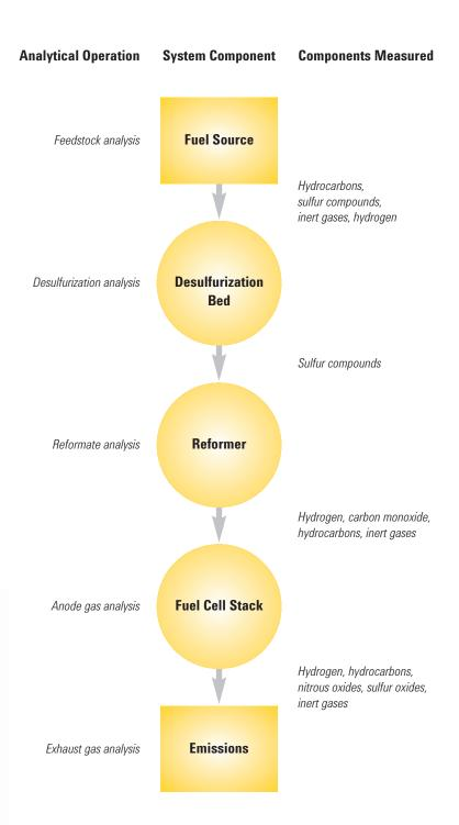
Fuel cell performance and efficiency can be evaluated by chemical measurements at key points in the sample stream, from composition of the feedstock to the emissions. Measurement of the chemical composition of primary reactants to the fuel cell allows precise determination of stack efficiency. It can also help you optimize the design of sub-assemblies and verify the overall system design by providing you with information for accurate mass balances.
