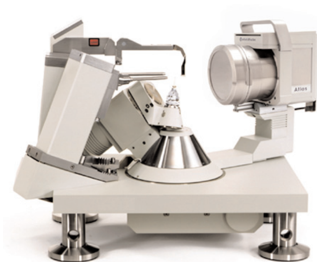
Figure 1. 4-circle kappa Gemini platform fitted with an Atlas CCD detector and co-mounted molybdenum Enhance and copper Enhance X-ray sources.
