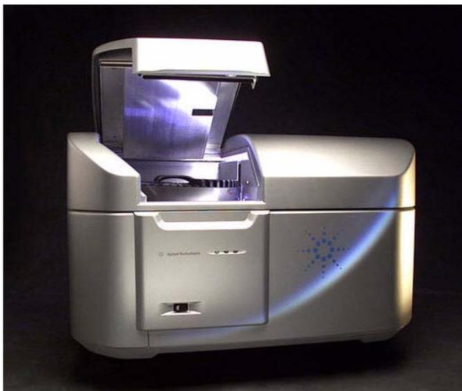
**Figura 1** Scanner per microarray Agilent G2565CA
