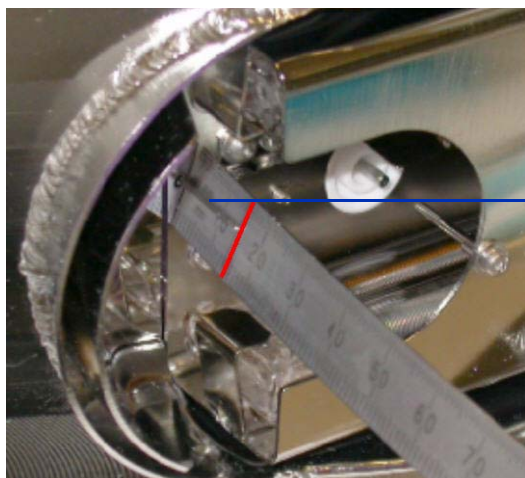
Figure 2 Installing the thermocouple probe and 15 mm adjustment
