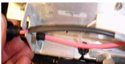
Figure 11 Connecting the HV PCA to the chassis.
