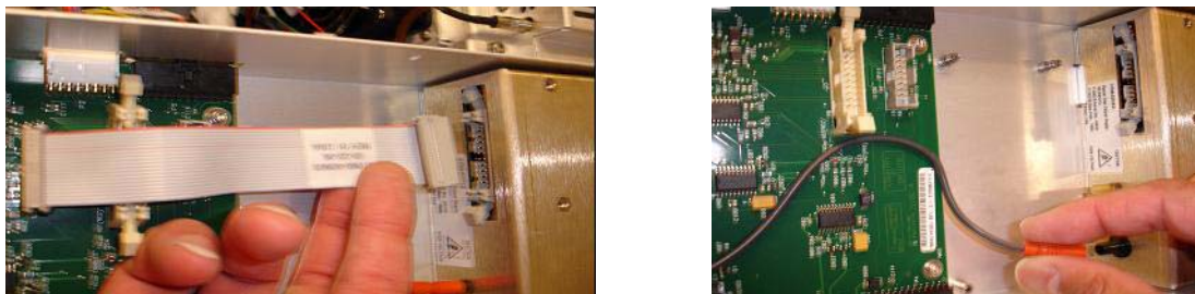
Figure 5 Disconnecting the Vcap/Vchamber power supply from the valve PCA (left) and the Vcap/Vchamber.
