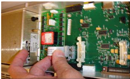
Figure 6 Connecting the valve PCA to the multimode HV power supply.
