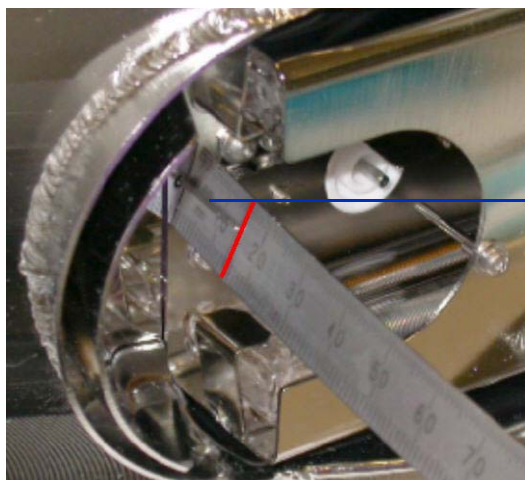
Figure 2 Installing the thermocouple probe and 15 mm adjustment
