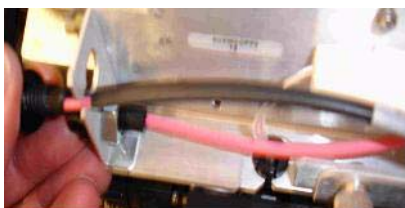
Figure 11 Connecting the HV PCA to the chassis.
