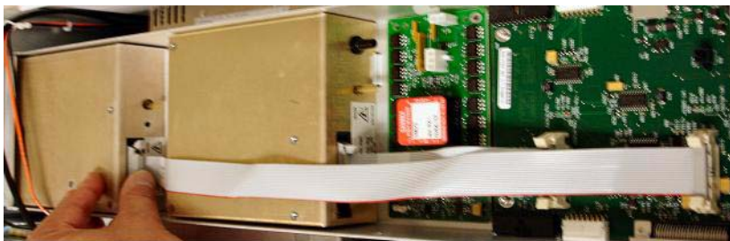
Figure 9 Connecting the APCI HV power supply to the valve PCA.
