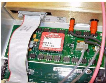
**Figure 8** Connecting the Vcap and Vchamber cables to the power supply.
