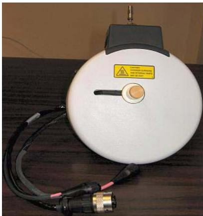
**Figure 17** Multimode Spray Chamber
