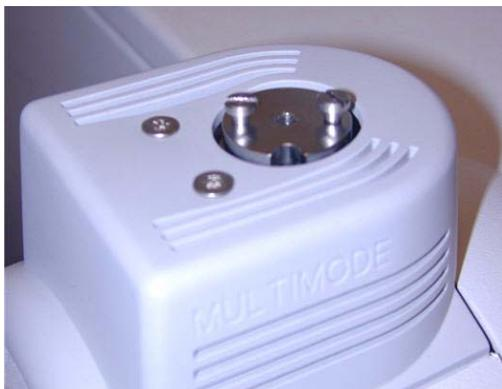
**Figure 19** No nebulizer on top of the multimode source
