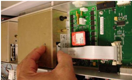
**Figure 7** Connecting the valve PCA to the Vcap/Vchamber power supply.
