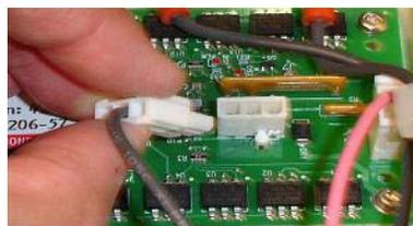
**Figure 11** Connecting the HV PCA to the chassis.
