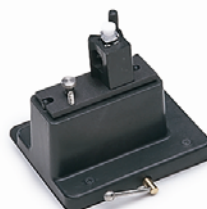
Figure 2 the standard Eclipse cell holder. The sample used was fluorescent ink diluted to give reasonable scale readings in a 3ml cuvette. The same holder is used for the microvolume cuvette.
