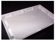
The Porvair 30uL shallow-well microplates are available in fluorescence grade white, black and clear designs. The design incorporates a shallow internal base yet it is stiff and strong enough for robotics applications. The wells hold just over 30uL to full and can be used with smaller volumes down to about 20uL.
