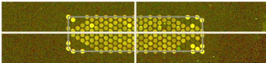
**Figure 35** Final position of main grid on 244k microarray
