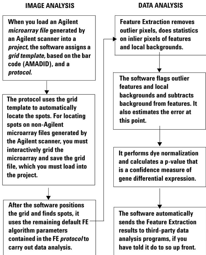
**Figure 1** Process flow for Feature Extraction
