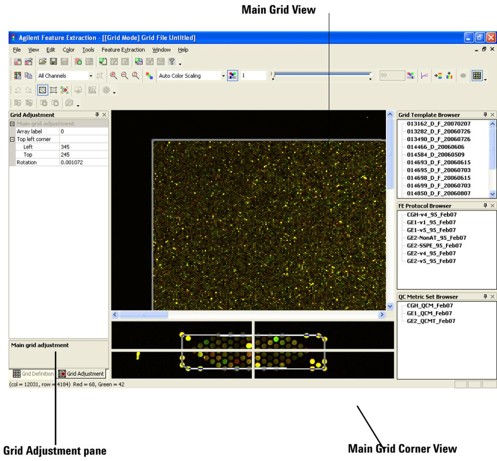
**Figure 29** Main Grid View for Agilent image with Agilent grid template
