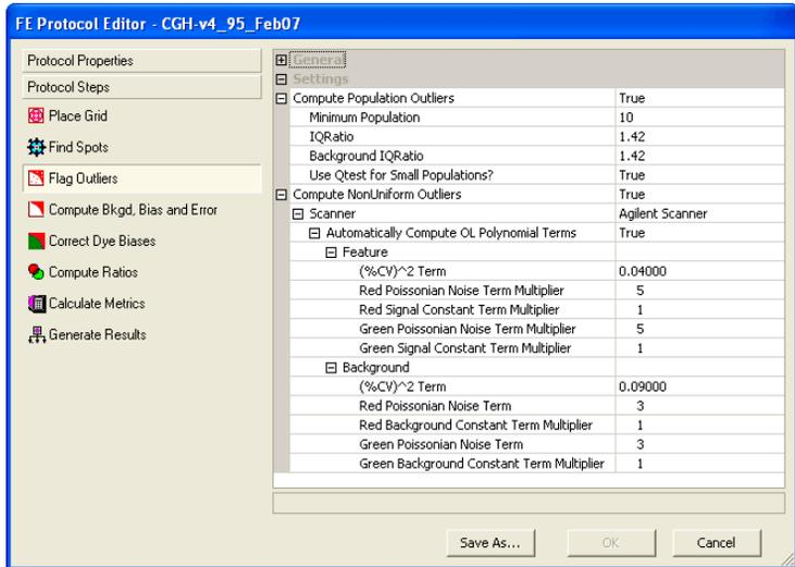
The polynomial equation for the noise model is still used, but rather than entering values for the A, B and C terms as in the “False” case, you enter the values for multipliers for the B and C terms in both color channels (2-color) or one channel (1-color).
