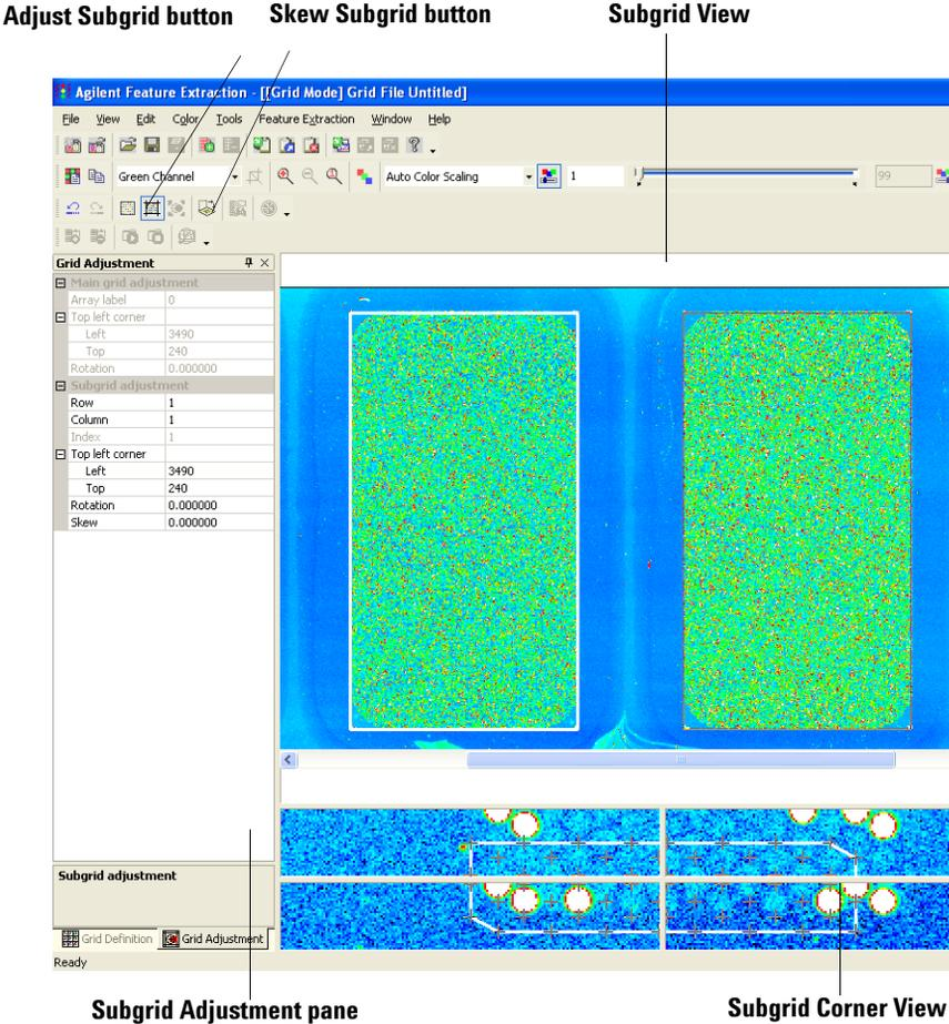
**Figure 37** Subgrid View with Grid Adjustment pane for a 1-color 4X44k multiplex (formerly known as multipack) microarray
